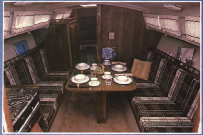
The traditional interior is shown with the table fully opened. The table also folds in half or stores flat against the bulkhead. The hull liner and overhead are attractive textured molded fiberglass. A wide choice of available fabrics and upholstery allow you to create a distinctive interior. All trim and cabinetry are teak.
