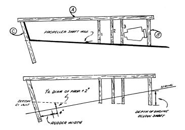
Fig.2 Method of Locating Shaft Hole
