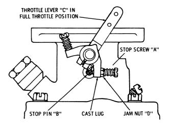
Fig.69 Carburetor - Adjustments
