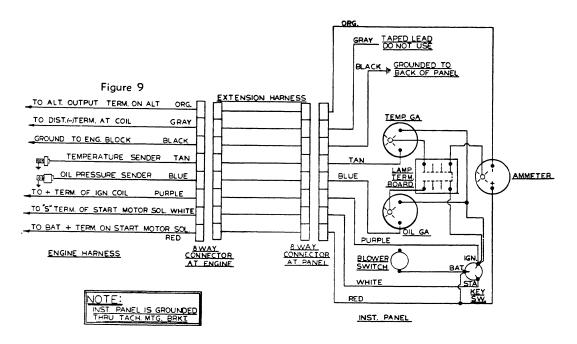
**Electric Instrument Panel less Tachometer**
