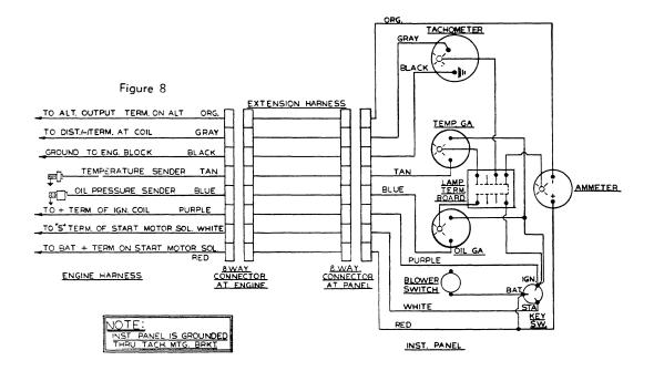
Electric Instrument Panel with Tachometer
