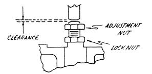
Fig.70 Valve Tappet - Adjustment
