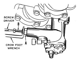
Fig.76 Oil Pressure Regulator - Adjustment
