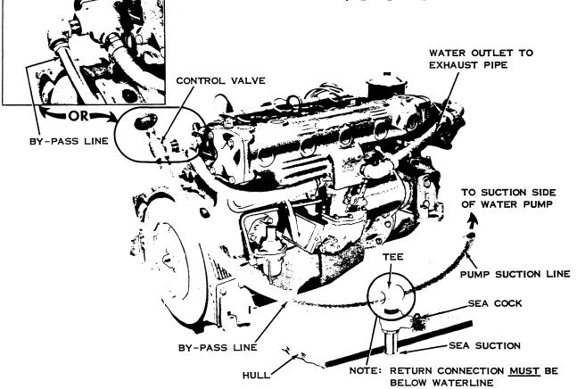
Fig. 11 Methods of Engine Temperature Control
