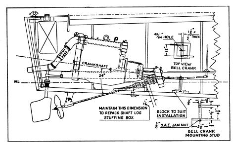
Fig.16 Typical V-Drive Layout
