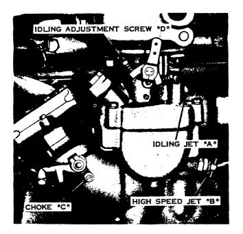
Fig.68 Carburetor - Adjustments
