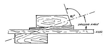
Fig.4 Method of Drilling Shaft Hole
