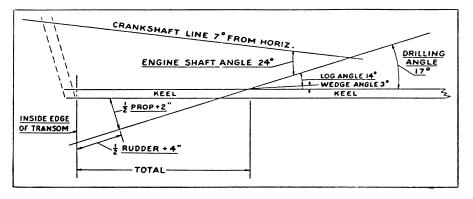
Fig. 12 Typical Shaft Location
