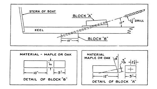
Fig. 14 Drill Block Details
