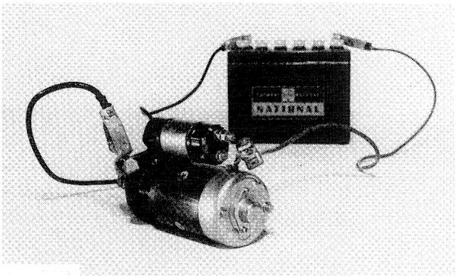
[A] Electrical connections for testing motor
