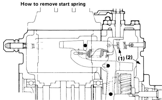
1. Detach Start Spring on the Side of Gear Case
