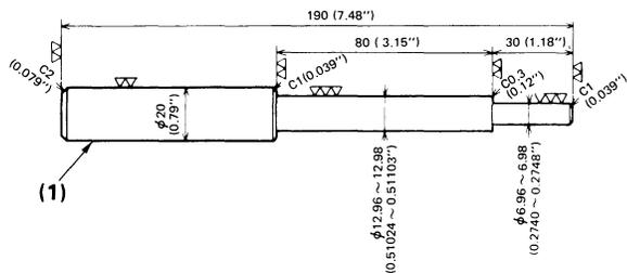
**(B) Finishing size of inlet valve guide**
