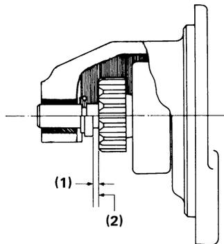
[A] Adjustment of pinion gap
