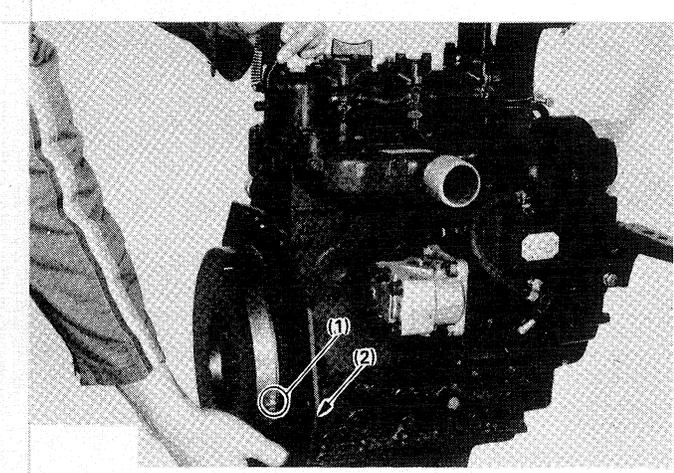
Adjustment of injection timing
