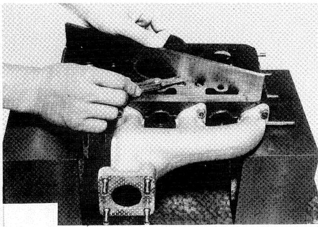
How to check cylinder head surface
