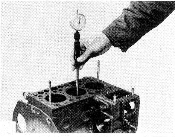
Measuring points of cylinder liner
