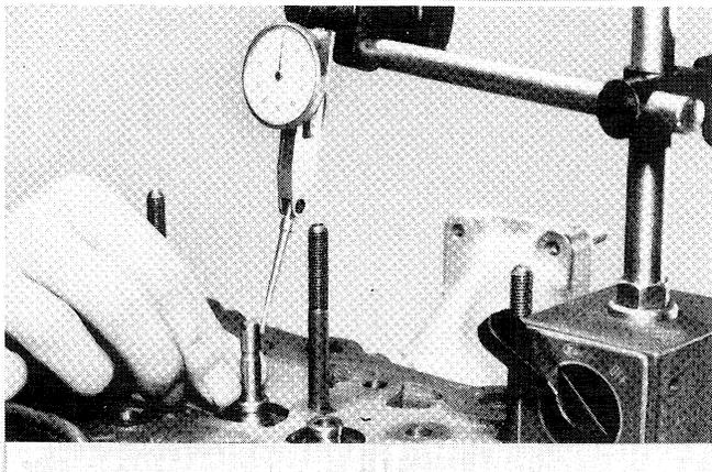
Finishing size of inlet valve guide
