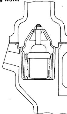
Temperature sensor of wax pellet type thermostat
