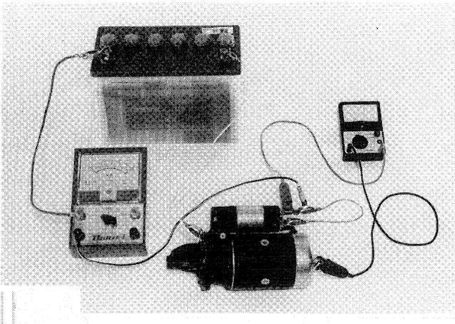
[A] Electrical connections for no-load testing.
