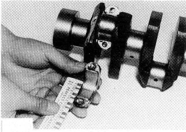
Crank pin measuring points
