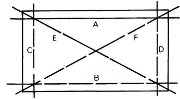
**CHECKING FLAW OF CYLINDER HEAD SURFACE**
