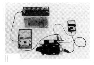
[A] Electrical connections for no-load testing.
