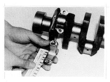
Crank pin measuring points
