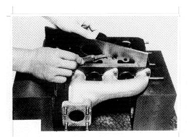
How to check cylinder head surface
