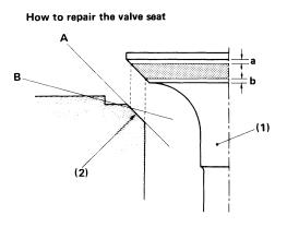
A 45° cutter (1) Valve B 15° cutter (2) Corrected surface of valve seat
