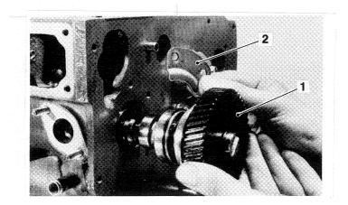
1. Fuel Camshaft Assembly 2. Fuel Camshaft Stopper
