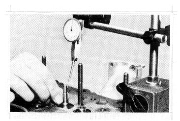
Finishing size of inlet valve guide
