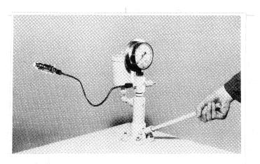
CHECKING FUEL TIGHTNESS OF NOZZLE VALVE SEAT
