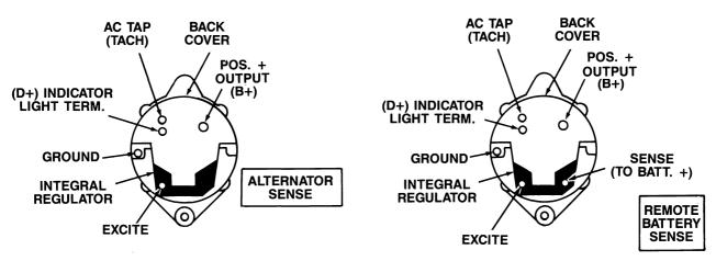
ALTERNATOR TERMINAL IDENTIFICATION (INTEGRAL REGULATOR)
