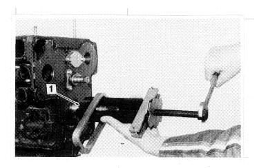
1. 13T Gear (Crank Gear)
