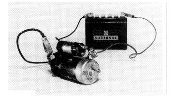
[A] Electrical connections for testing motor
