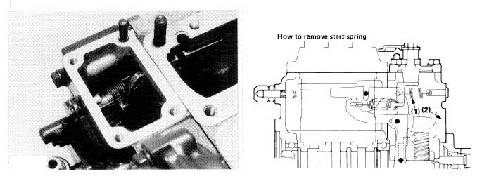
1. Detach Start Spring on the Side of Gear Case 2. Gear Case
