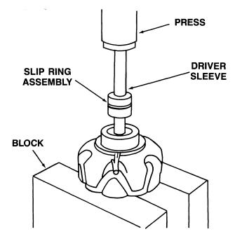
INSTALLING SLIP RING ASSEMBLY
