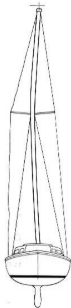
Starboard lower too tight Port lowers too loose
