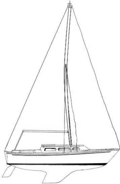
Aft lower shrouds too tight Forward lowers too loose
